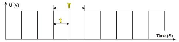
Duty cycle = t / T, when t is the half of the entire period Duty cycle=0.5 (50%). This case is shown on the figure above. The Duty cycle equal to 50% is the most common case in the practice when the signals from different sensors are simulated.
