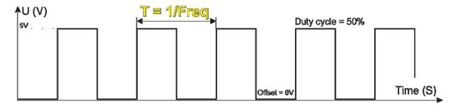
Interval of time in which some event repeats is called period. In the SI system the period is marked with T and it is measured in seconds [s]. The
