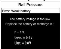
Solution: Recharge or replace the battery!
