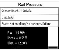
You can see the actual pressure as well as sensor and battery voltages during cranking. If the engine cannot start, you could directly/indirectly find the reason for that.
