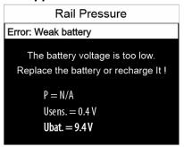
Solution: Recharge or replace the battery!
